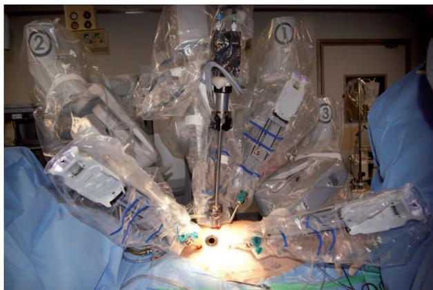
Fig. 2 - External aspect of the operative field: DaVinci® robotic system connected to trocars
